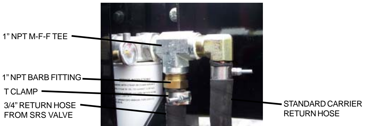
Figure 6 - Hydraulic Tank Return Lines
